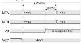
Figure 5: Intersection from main supply VCC to auxiliary supply VB.
