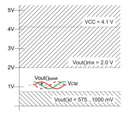
Figure 1: Permissible maximum output voltage range and example of typical output voltage.
