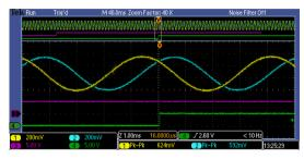
Figure 2: Regular Gray code output at MTA (CH3, magenta) and MTB (CH4, green) during normal operation; shown with PS\_M (CH1, yellow) and PC\_M (CH2, blue).
