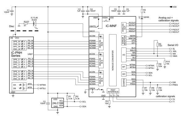
Figure 7: Application example of absolute encoder circuit.
