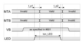
Figure 6: MTA and MTB output validity depending on LED flash.
