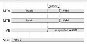
Figure 4: Outputs MTA and MTB operated from auxiliary supply VB.
