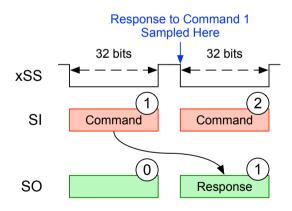
Figure 40: SPI Position Read
