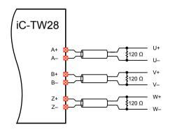
Figure 30: UVW Output Connections
