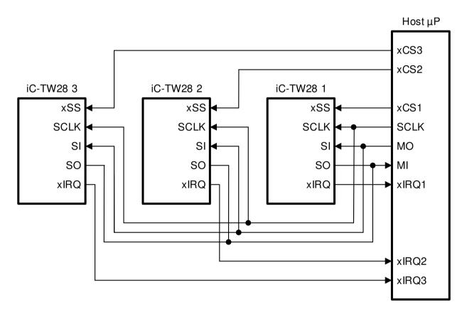
Figure 45: SPI Bus Connection of Multiple iC-TW28s
