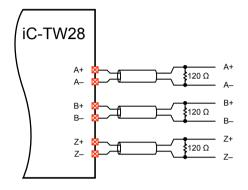
Figure 17: ABZ Output Connection
