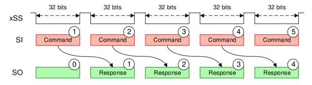
Figure 21: SPI Overlapped Packet Structure
