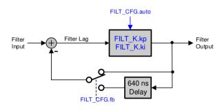
Figure 39: Signal Path Filter
