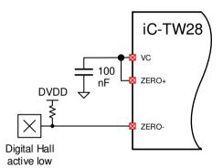
Figure 15: Digital Index Sensor Connection
