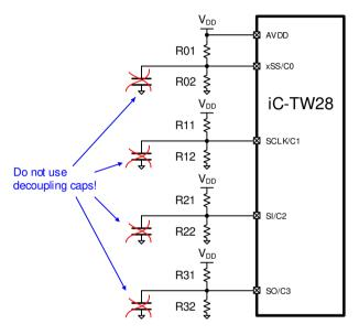
Figure 19: Pin Configuration Resistors
