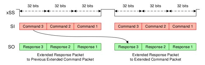
Figure 47: Extended Communication Packet Structure With Chained iC-TW28s
