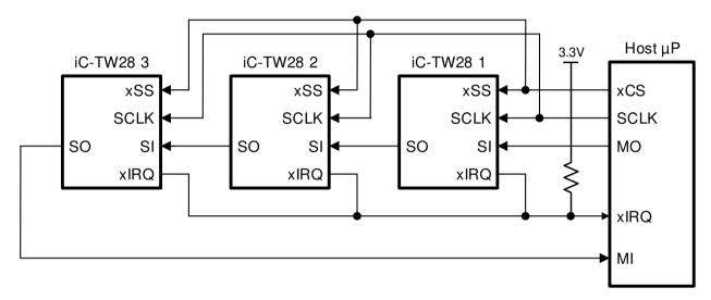
Figure 46: Chained Connection of Multiple iC-TW28s
