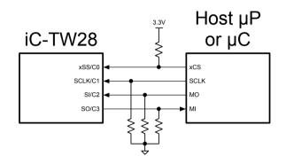
Figure 20: SPI Port Connection
