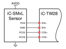
Figure 13: Magnetic Sensor Connection
