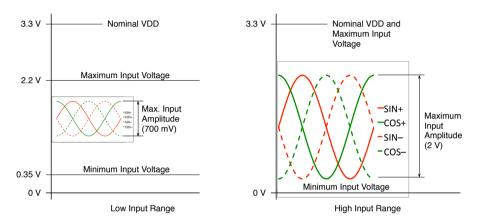
Figure 1: Differential Input Amplitude Ain()diff: Max(SIN+ - SIN-) or Max(COS+ - COS-)
