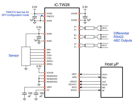
Figure 12: Typical Electrical Connections For Hosted Application
