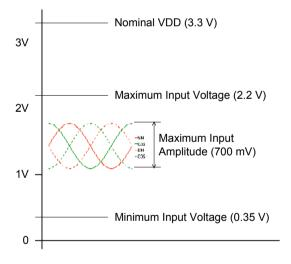
Figure 27: Low Input Range Signals
