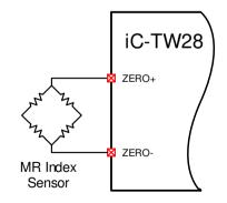
Figure 16: Analog Index Sensor Connection
