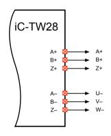
Note that the UVW outputs are inverted; set the uvwpol bit to provide normal UVW output polarity. The apol, bpol, zpol, abzdir, and uvwdir bits can be used as explained previously to set the desired polarities and directions of the ABZ and UVW outputs.
