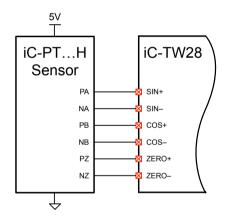
Figure 14: Optical Sensor Connection
