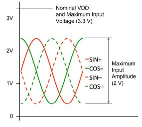
Figure 28: High Input Range Signals
