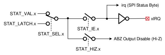
Figure 33: Single Condition Status and Fault Logic
