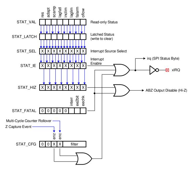
Figure 34: iC-TW28 Status and Fault Logic
