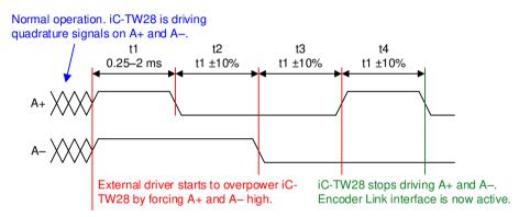
Figure 24: Encoder Link Activation Sequence
