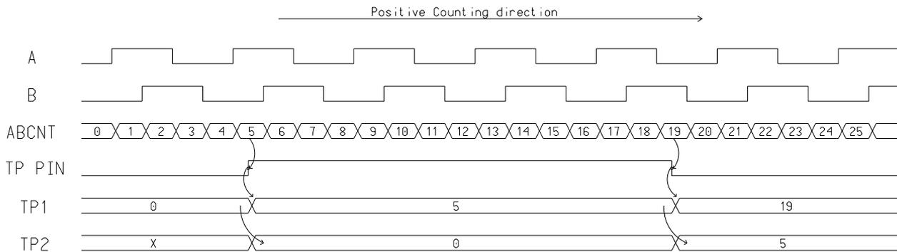
Figure 7: Function of TPI pin when TPCFG=11
