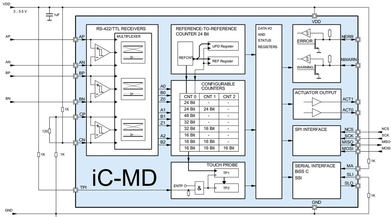
Figure 13: SPI only operation with unused constant pulled index input
