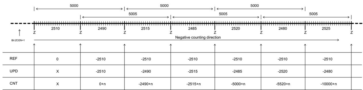
Figure 6: REF and UPD registers in negative direction
