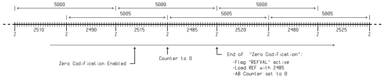
Figure 5: Zero-Codification: reference position acquisition
