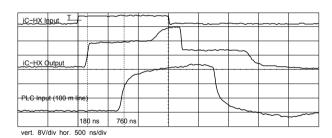
Figure 4: Pulse transmission and transit times
