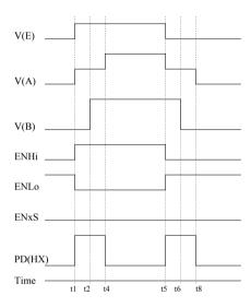
Figure 6: Power dissipation  ${\rm P_D(HX)}$  without iC-xSwitch
