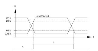
Figure 1: Reference levels for delays
