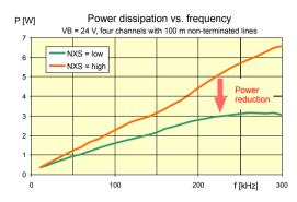
Figure 8: Power dissipation with and without xSwitch-Mode
