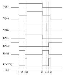
Figure 7: Power dissipation  $P_D(\mathrm{HX})$  with iC-xSwitch
