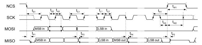
Figure 1: Timing SPI Interface
