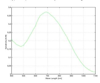
Figure 3: Spectral sensitivity of the photodiode
