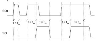
Figure 7: Rise and fall delay
