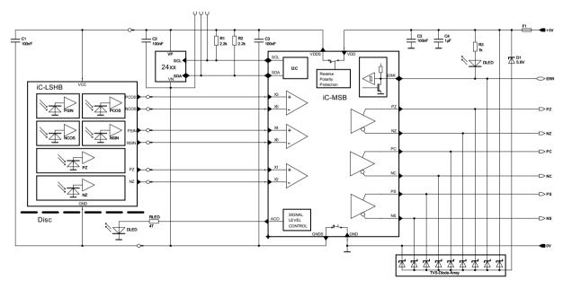
Figure 2: Example of sine encoder with 1 Vpp output
