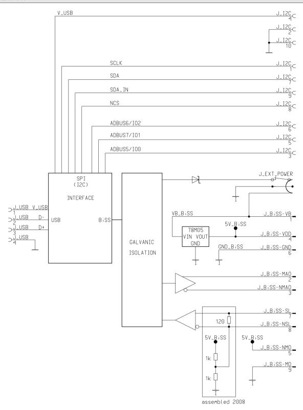
Figure 2: Power supply routing of MB3U-I2C
