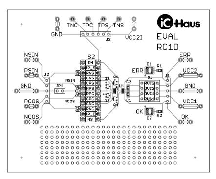
Figure 7: Layout of component side
