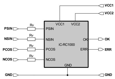
Figure 3: Overvoltage protection with external resistors
