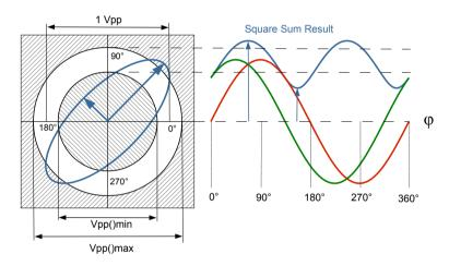
Figure 5: Monitoring of Lissajous figure regarding phase error tolerance
