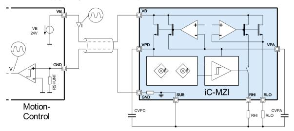
Figure 9: Sourcing and sensing the iC-MZI as a two-wire sensor
