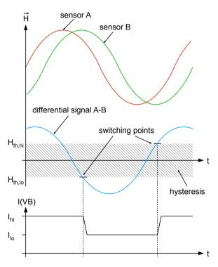
Figure 2: Signal transfer characteristics
