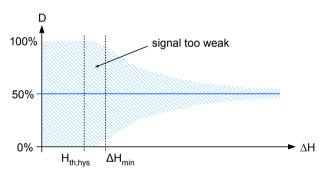
Figure 5: Duty-cycle as a function of  $\Delta H$
