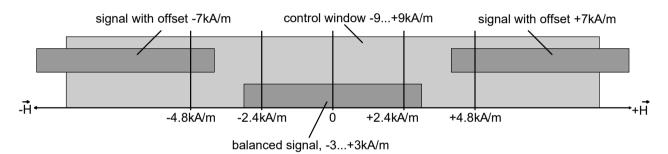
Figure 6: Adjustment range and starting values
