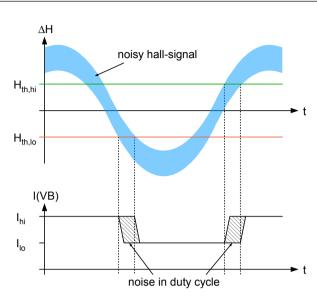
Figure 4: Effect of noise on output duty-cycle
