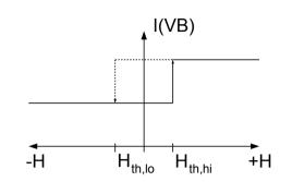
Figure 1: Current level switching vs. magnetic field difference
