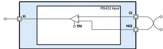
Figure 6: Equivalent circuit of RS-422 receiver
