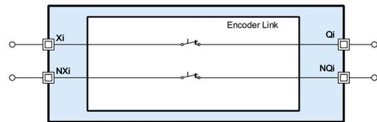
Figure 3: Equivalent circuit of 1 channel (2 lines) in *Encoder Link State*
