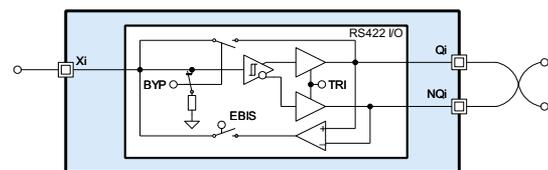
Figure 4: Bidirectional channel
