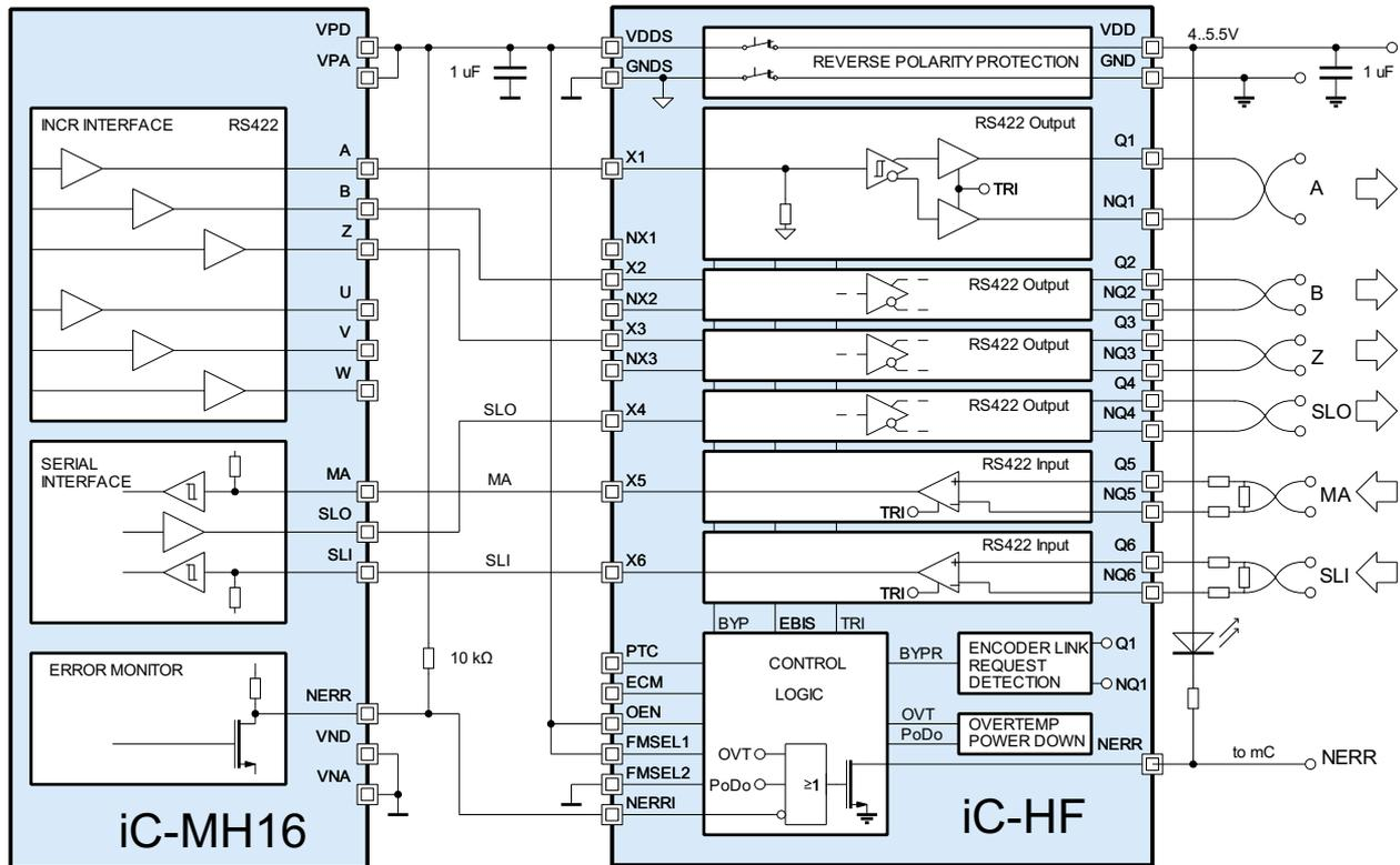
Figure 30: Example application with iC-MH16 in A/B/Z and BiSS/SSI mode
