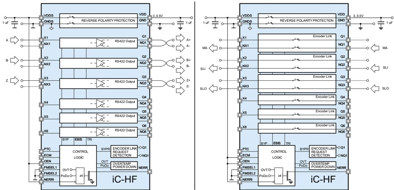
Figure 36: iC-HF with BiSS + A/B/Z using only 8 lines
