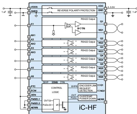
Figure 8: *A/B/Z and U/V/W* mode, 6 channel line driver
