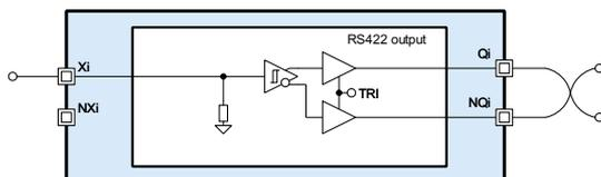
Figure 2: Equivalent circuit of unidirectional RS-422 driver channel
