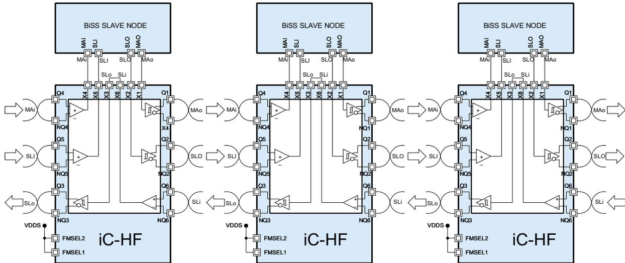
Figure 14: Several slave nodes in *BiSS bus structure*
