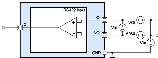
Figure 24: RS-422 input sensitivity
