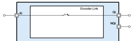
Figure 7: Equivalent circuit of one line in *Encoder Link State*
