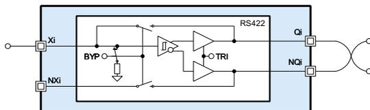
Figure 1: Unidirectional channel
