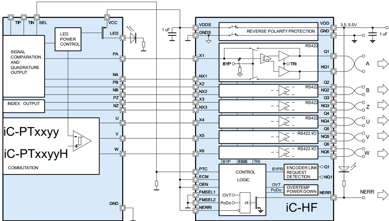
Figure 28: Example application of iC-PTxxyy/ iC-PT-Hxxyy in A/B operation x1 interpolated with iC-HF
