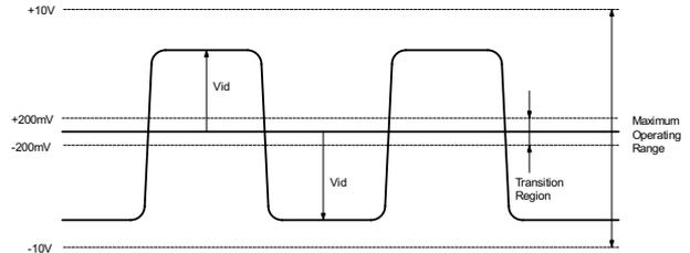
Figure 25: RS-422 input maximum and minimum operating voltages
