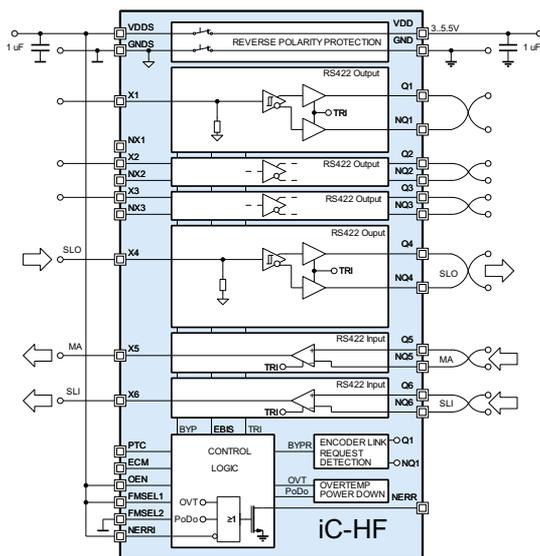
Figure 10: A/B/Z and BiSS/SSI mode, 3 channels line driver
