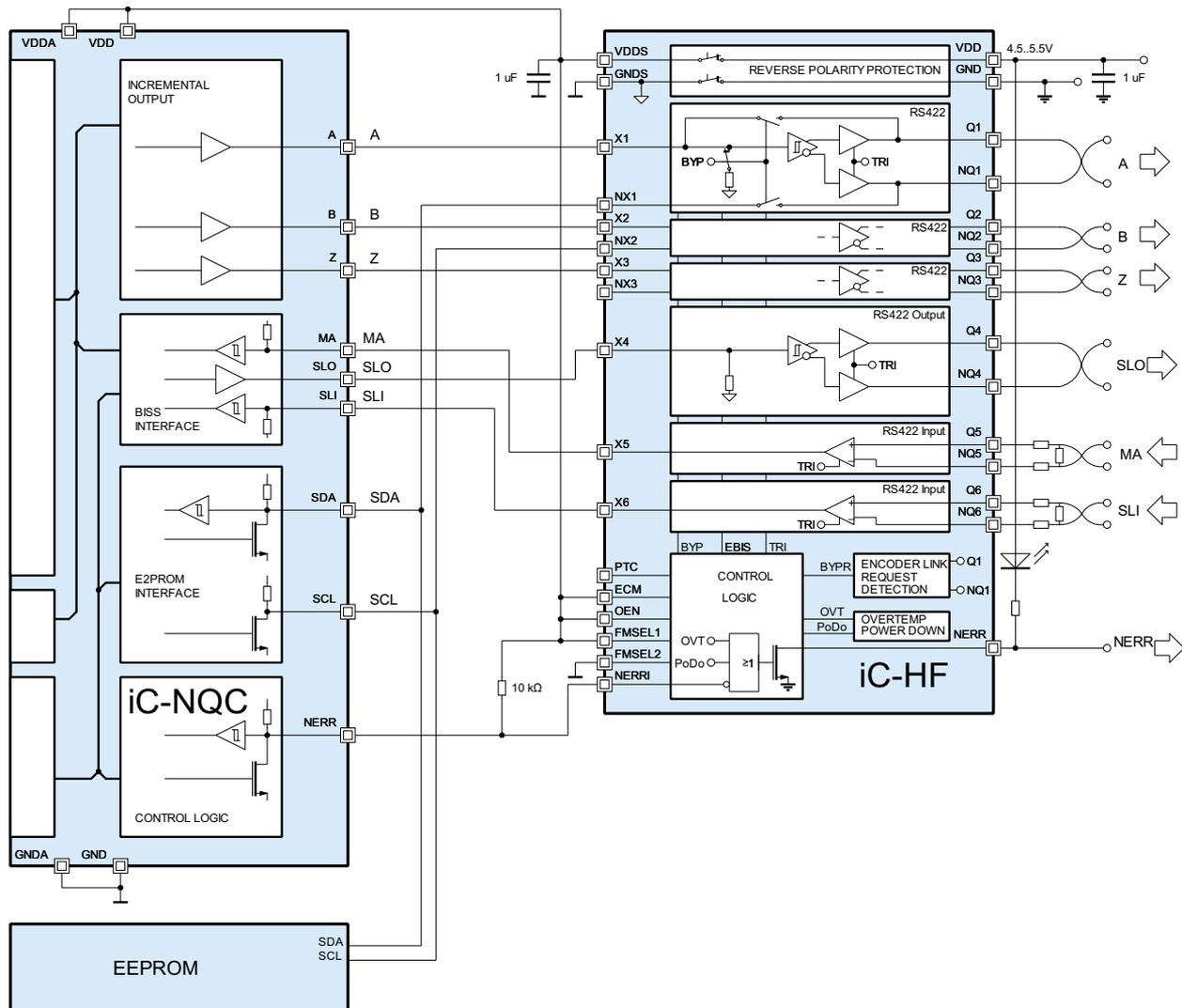
Figure 35: Example application of iC-NQC with iC-HF
