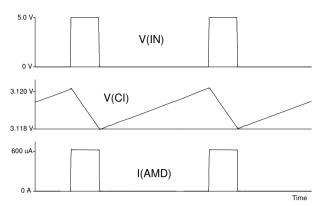
Figure 4: Steady-state APC, f(IN) = 100 kHz (1:4), CI = 470 nF, RSET = 10 k $\Omega$
