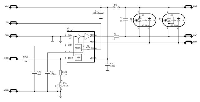
Figure 12: Schematic diagram of the Demo Board
