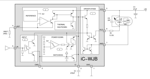
Figure 1: Circuit diagram for LD models with a common cathode
