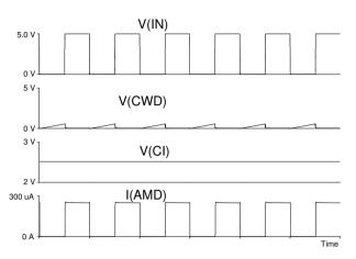
Figure 8: Watchdog, CWD open, f(IN) = 100 kHz(1:1), CI = 470 nF, RSET = 10 k $\Omega$
