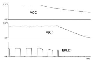
Figure 7: Turn-off behaviour, f(IN) = 100 kHz (1:1), CI = 470 nF, RSET = 10 k $\Omega$
