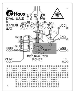
Figure 13: Demo Board (components side)
