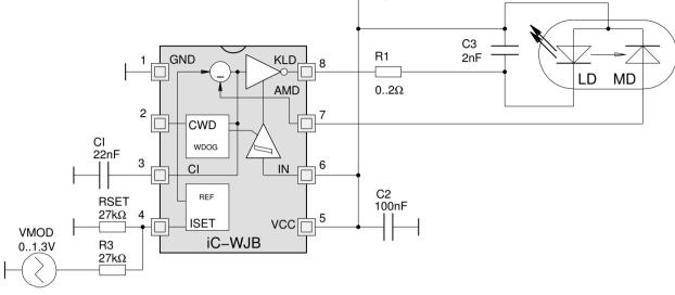
Figure 11: Analogue modulation during CW operation
