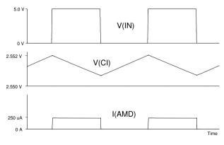
Figure 3: Steady-state APC, f(IN) = 100 kHz (1:1), CI = 470 nF, RSET = 10 k $\Omega$
