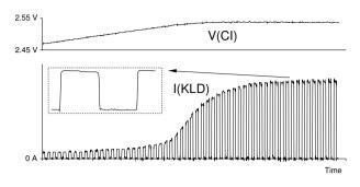
Figure 6: Turn-on behaviour, detailed view f(IN) =100 kHz (1:1), CI = 470 nF, RSET = 10 k $\Omega$
