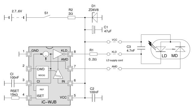
Figure 10: CW operation via cable plus protective circuitry
