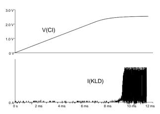
Figure 5: Turn-on behaviour, f(IN) = 100 kHz (1:1), CI = 470 nF, RSET = 10 k $\Omega$
