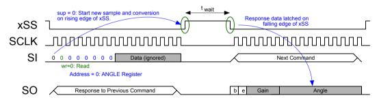
Figure 6: Reading the ANGLE register
