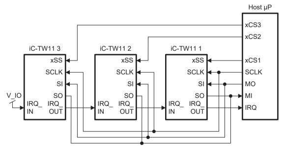
Figure 9: SPI bus connection of multiple iC-TW11s
