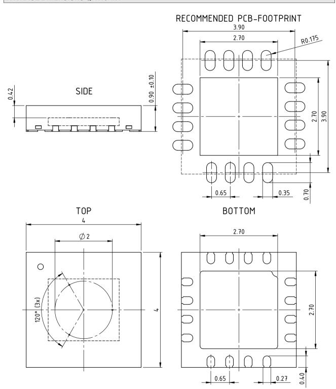
All dimensions given in mm. Tolerances of form and position according to JEDEC M0-220. Positional tolerance of sensor pattern: ±0.1mm / ±1° (with respect to backside pad). dra\_qfn16-4x4-2\_tw11\_c2\_pack\_1, 15:1
