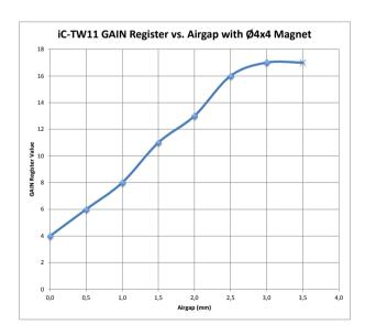
Figure 8: Typical Hall array gain vs. airgap
