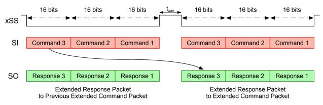
Figure 11: Extended communication packet structure with chained iC-TW11s
