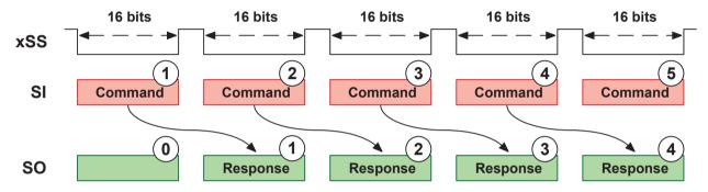
Figure 5: SPI overlapped packet structure
