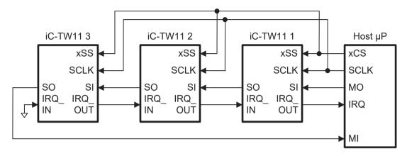
Figure 10: Chained connection of multiple iC-TW11s
