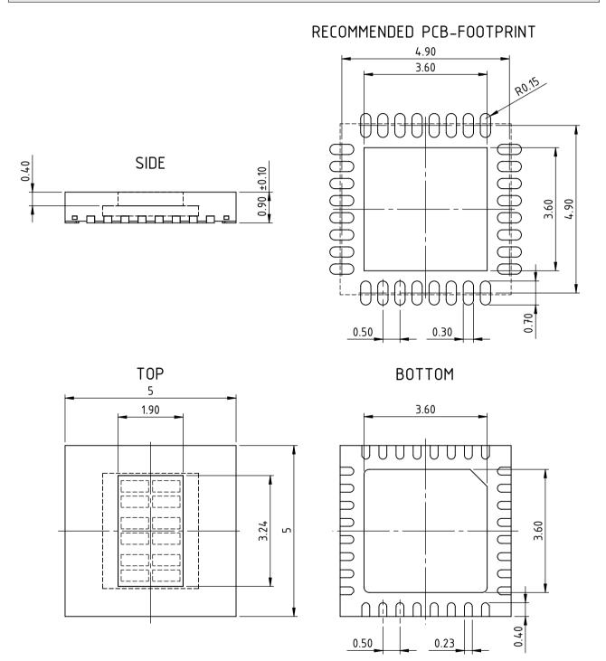
All dimensions given in mm. Tolerances of form and position according to JEDEC MO-220. Tolerance of sensor pattern:  $\pm 70\mu$ m /  $\pm 1^{\circ}$  (with respect to center of backside pad). Maximum molding excess  $\pm 20\mu$ m /  $-75\mu$ m versus surface of glass/reticle.
