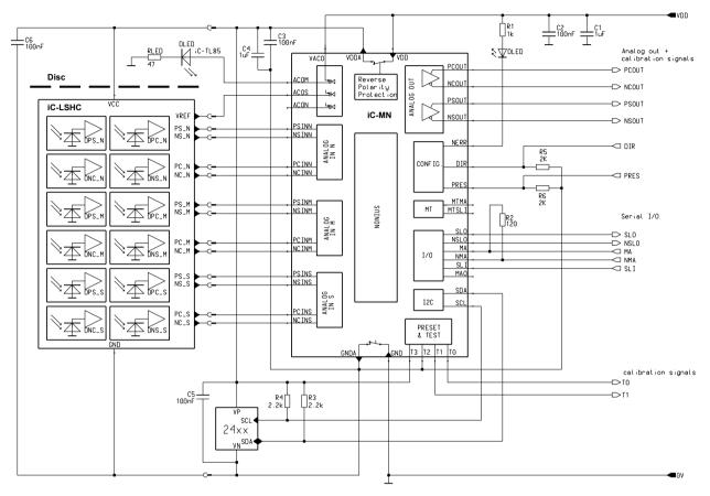
Figure 1: Application example of absolute encoder
