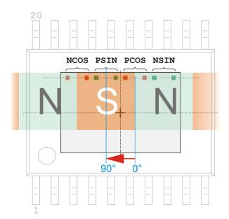
Figure 6: Position of the magnetic target at 90 ° electrical position. Center of south pole is aligned to the PSIN sensor pair
