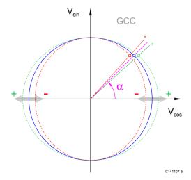
Figure 16: Effect of the amplitude ratio
