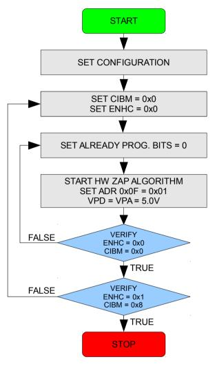
Figure 26: Programming algorithm
