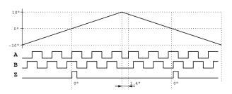
Figure 19: Quadrature signals for rotating direction reversal (hysteresis 1.4°)
