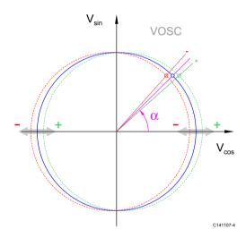
Figure 15: Effect of the cosine offset setting
