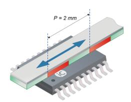
Figure 2: Typical arrangement of a magnetic tape to iC-MHL100
