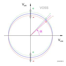
Figure 14: Effect of the sine offset setting
