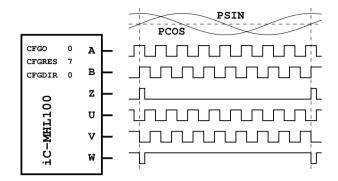
Figure 20: ABZ differential incremental signals
