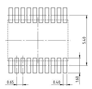
All dimensions given in mm. Tolerances of form and position according to JEDEC MO-153.
