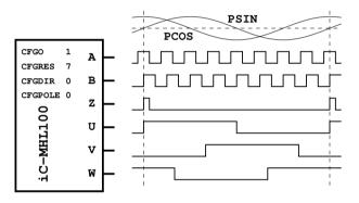
Figure 21: ABZ incremental / UVW commutation signals
