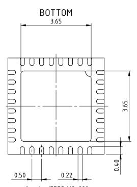
All dimensions given in mm. Tolerances of form and position according to JEDEC M0-220. Tolerance of sensor pattern:  $\pm 0.10$ mm /  $\pm 1^{\circ}$  (with respect to center of backside pad).
