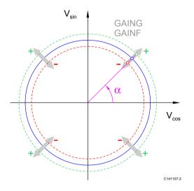
Figure 13: Effect of gain settings GAING and GAINF
