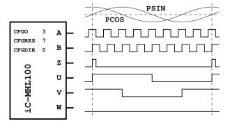
Figure 23: ABZ incremental signals / period counter
