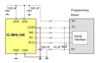
Figure 27: Recommended setup for external programming. A short low impedance path (shown in light red) must be provided directly from pin VZAP to pin VNA
