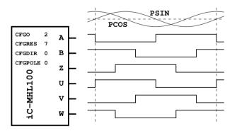
Figure 22: UVW differential commutation signals
