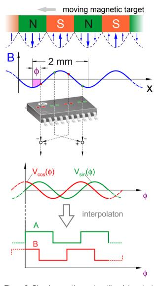
Figure 3: Signal generation and position data output
