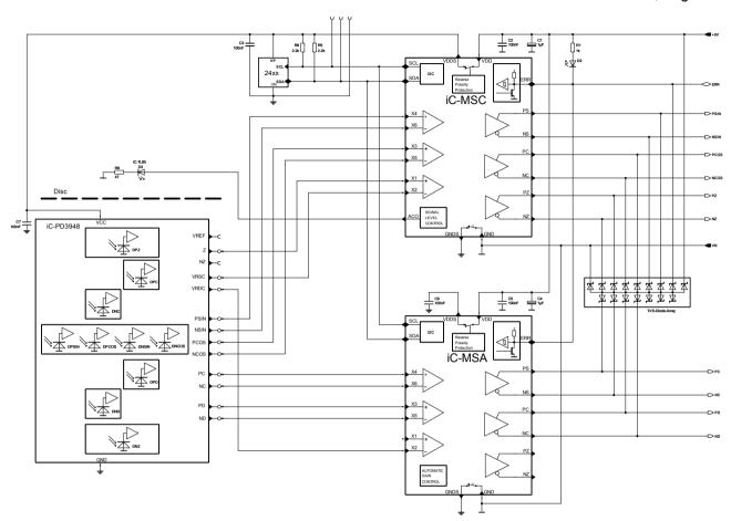
Figure 2: Application example motor feedback encoder utilizing iC-MSC and iC-MSA.
