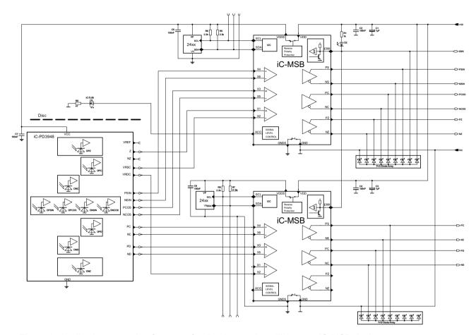
Figure 1: Application example of a motor feedback encoder utilizing two iC-MSB devices. Sine square plus cosine square LED power controlling by iC-MSB maintains the differential 1 Vpp signal of the S/C channel featuring 2048 CPR. The C/D channel with 1 CPR is initially also calibrated to 1 Vpp differential, but experiences variation due to LED power controlling. This variation can be neglected at speeds below 1,500 rpm, as iC-PD3948 does not run into cut-off frequency.
