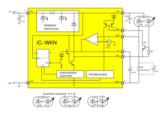
Figure 4: iC-WKN with selectable current limiter
