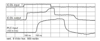
Figure 4: Pulse transmission and transit times
