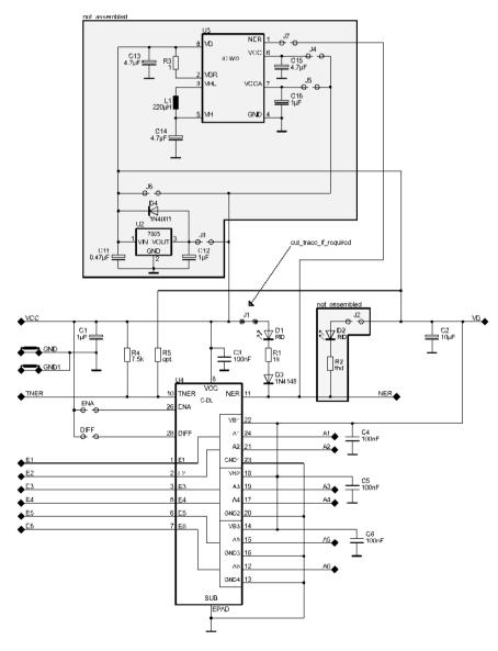
Figure 5: Circuit diagram of the evaluation board
