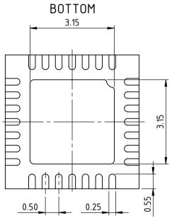
All dimensions given in mm. Tolerances of form and position according to JEDEC MO-220.
