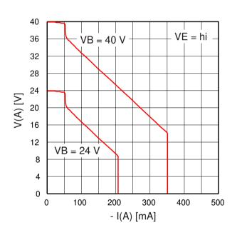
Figure 2: Load dependence of the output voltage (High-side stage)
