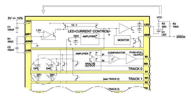
Figure 1: LED current control and monitoring.
