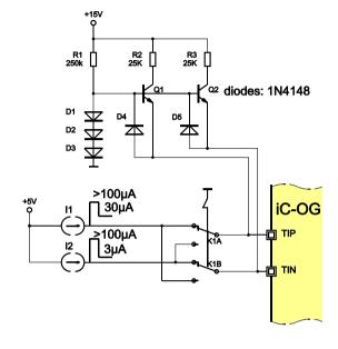
Figure 2: Wiring the test aid.
