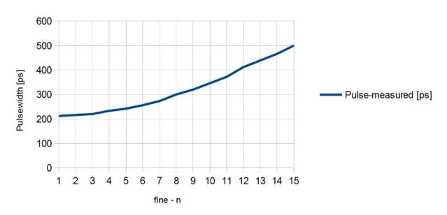
Figure 4: Setting the pulse width "fine"
