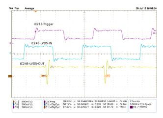
Figure 12: 100 MHz signal from iC213 and a long duty cycle > 97%
