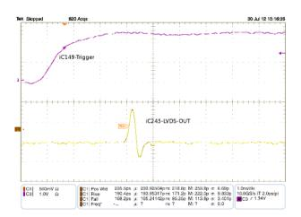
Figure 9: Minimum pulse width of 235 ps
