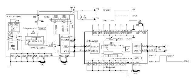
Figure 2: Block diagram of iC245 in connection with iC149
