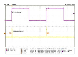
Figure 7: Maximum pulse width of 10.2 ns
