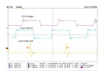
Figure 10: 100 MHz signal from iC213 and a short duty cycle < 3%
