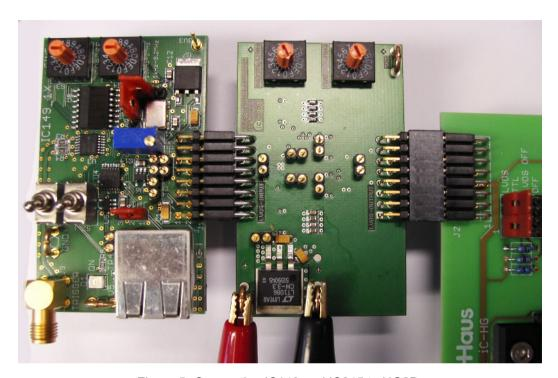
Figure 5: Connecting iC149 and iC245 to HG2D.
