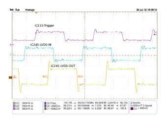
Figure 11: 100 MHz signal from iC213 and a duty cycle of 50%
