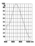
Figure 1: Relative spectral response
