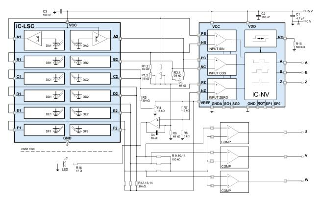
Figure 3: Optical encoder application example. Here, the sine-to-digital converter iC-NV is employed to output spike-free encoder quadrature signals featuring a minimum transition distance.
