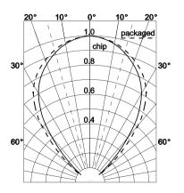
Figure 2: Typical directional characteristics
