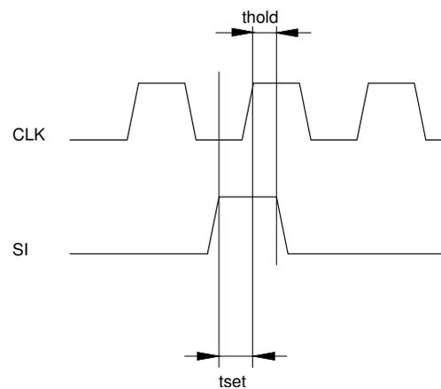
Figure 3: Timing diagram
