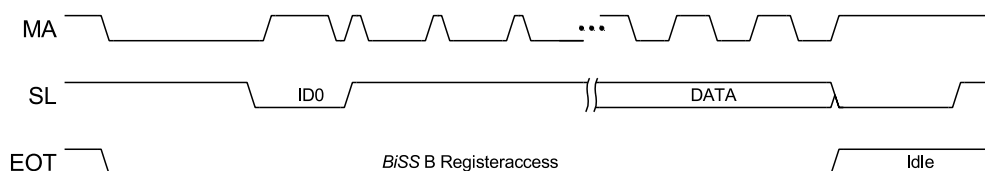
Figure 14: BiSS B register access (EN_MO = 0)
