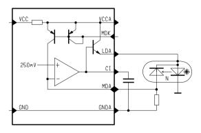
Figure 5: Operation of an N-type laser diode
