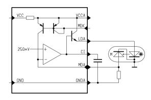
Figure 3: Operation of an M-type laser diode
