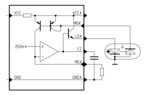
Figure 4: Operation of a P-type laser diode
