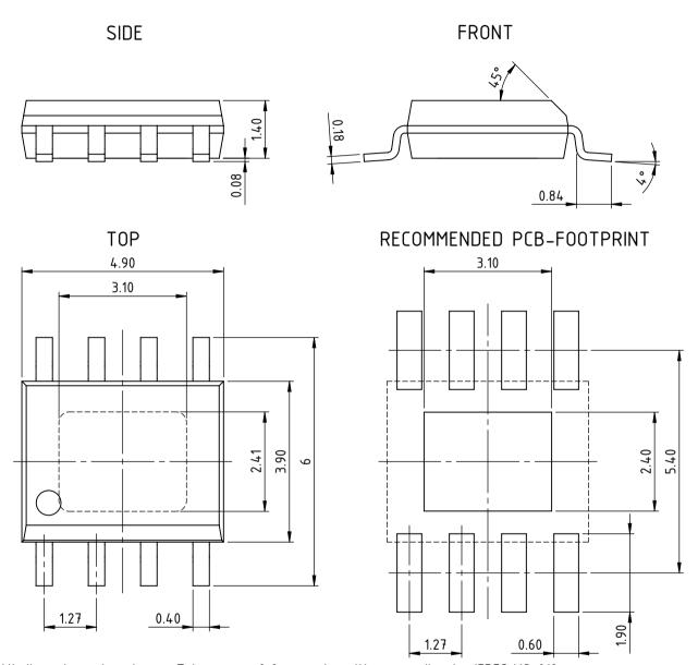
All dimensions given in mm. Tolerances of form and position according to JEDEC MS-012
