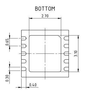
All dimensions given in mm. Tolerances of form and position according to JEDEC MO-229.
