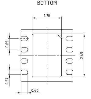
All dimensions given in mm. General tolerances of form and position according to JEDEC MO-229. Positional tolerance of sensor pattern:  $\pm70\mu\text{m}$  /  $\pm1^\circ$  (with respect to center of backside pad). Maximum molding excess  $\pm20\mu\text{m}$  /  $\pm75\mu\text{m}$  versus surface of glass. Small pits in the mold surface, which may occasionally appear due to the manufacturing process, are cosmetic in nature and do not affect reliability.
