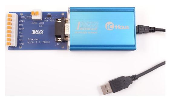
Figure 8: IC334 connected to iC-MB5 iCSY MB5U
