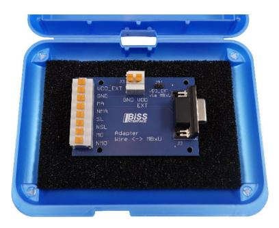
Figure 3: BiSS/SSI connection adapter iC334 - scope of delivery
