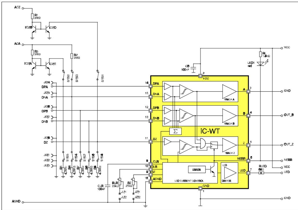
Fig. 2: Schematic diagram of the Demo Board
