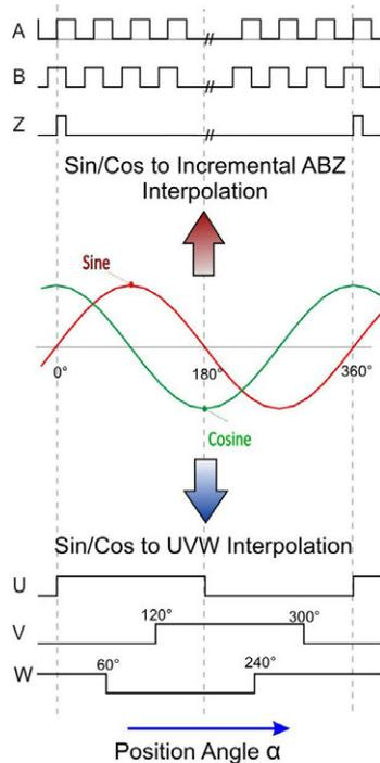
Fig. 2: Generating UVW and ABZ from Sine/Cosine.
