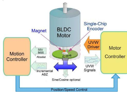
Fig. 3: Motor control with absolute magnetic encoder with outputs options.
