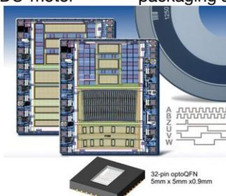
Fig. 4: Optical single-chip motor encoder ICs with UVW commutation.
