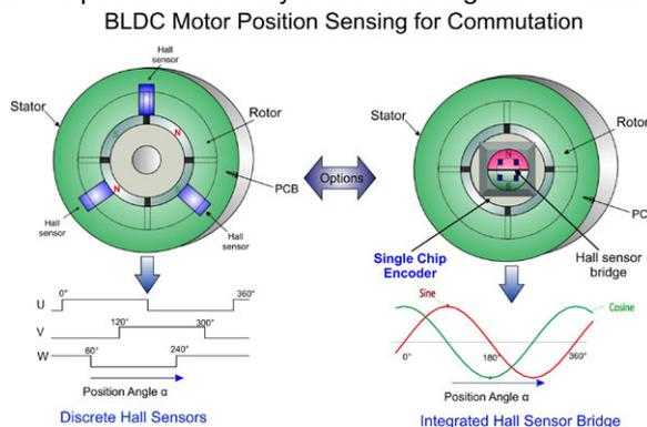
Fig. 1: Options of BLDC motor position sensing for commutation.
