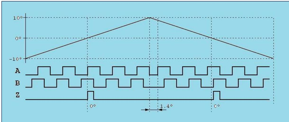
Figure 2: Timing diagram of the incremental encoder interface with A, B, and Z signals
