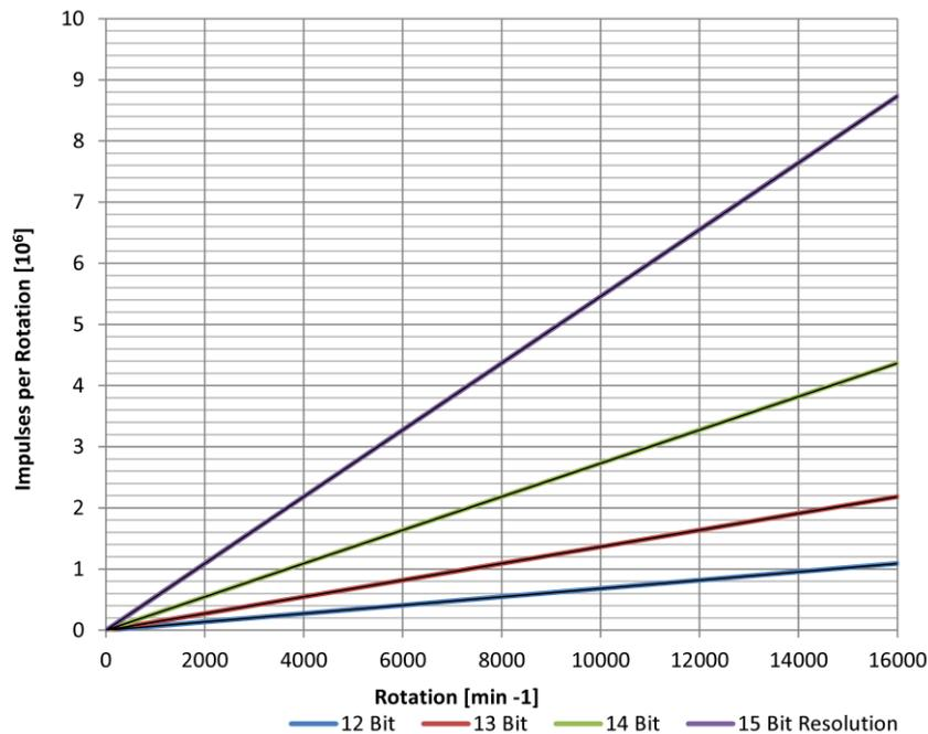
Figure 4b: Pulse rates depending on speed and resolution
