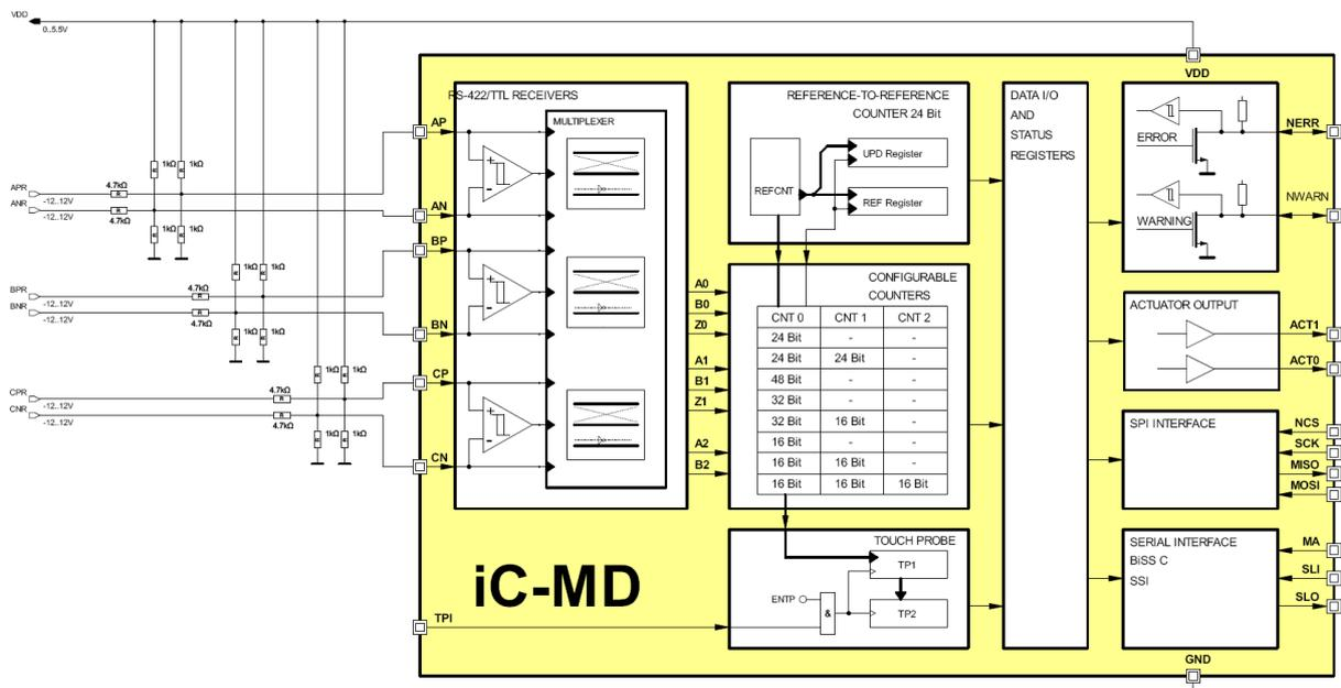
Figure 5: Three-channel incremental encoder interface with differential RS422 receivers
