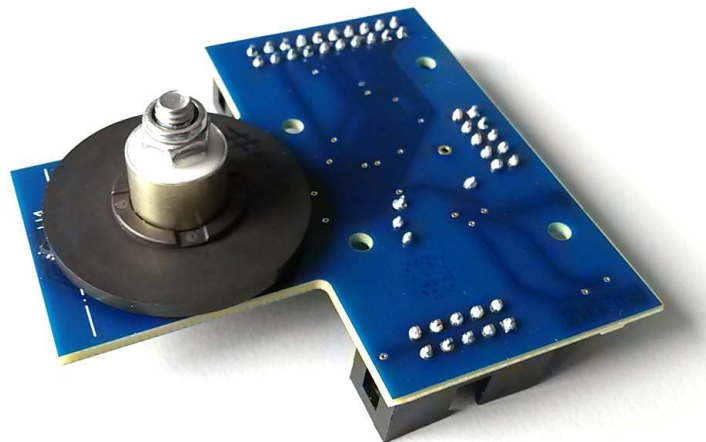
Figure 3: Bottom side with MU18S 30-32N magnetic code disc
