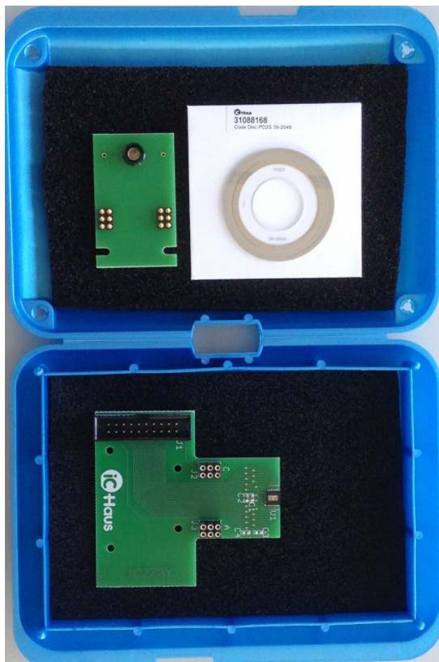
Figure 10: Evaluation kit. Scope of delivery: LED module, code disc, scanner module (hub not included)
