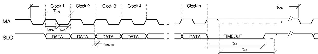
Figure 1: I/O interface timing with SSI protocol
