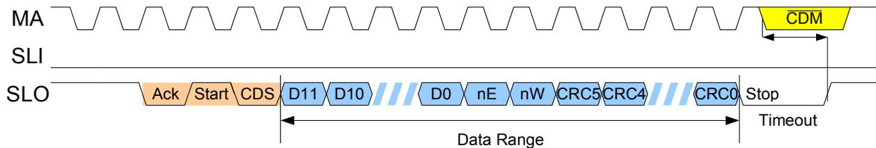
Figure 23: BiSS Interface Protocol Frame (Single Cycle Data SCD)
