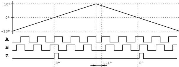
Figure 18: Quadrature signals for rotating direction reversal (hysteresis 1.4°)
