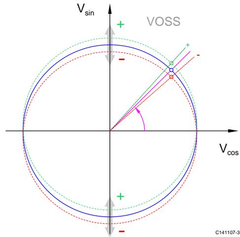
Figure 13: Effect of the sine offset setting
