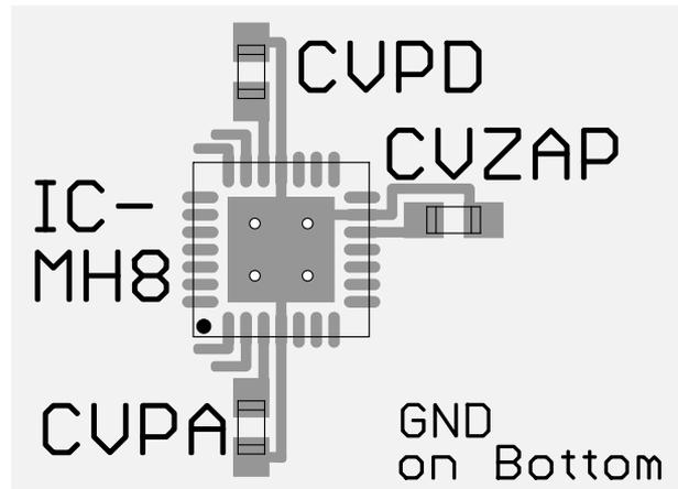
Figure 27: Example PCB layout showing low impedance connection of capacitors to supply voltages (VPA, VPD, VZAP) and common ground
