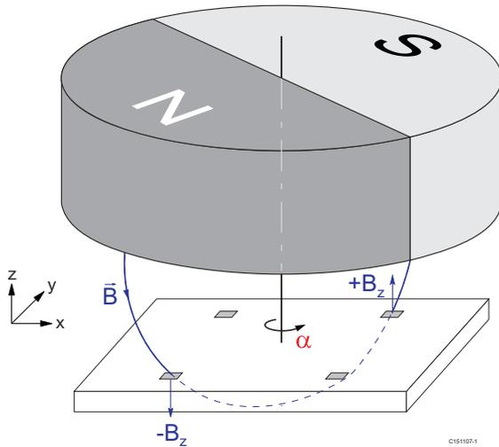
Figure 2: Sensor principle
