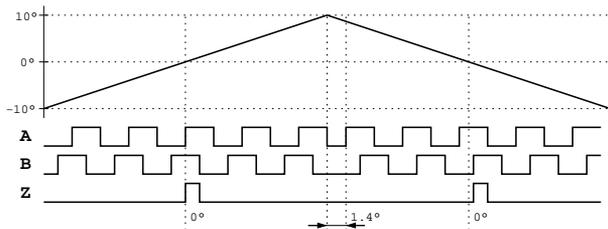
Figure 18: Quadrature signals for rotating direction reversal (hysteresis 1.4°)
