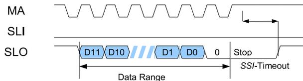
Figure 25: SSI protocol, data GRAY-coded
