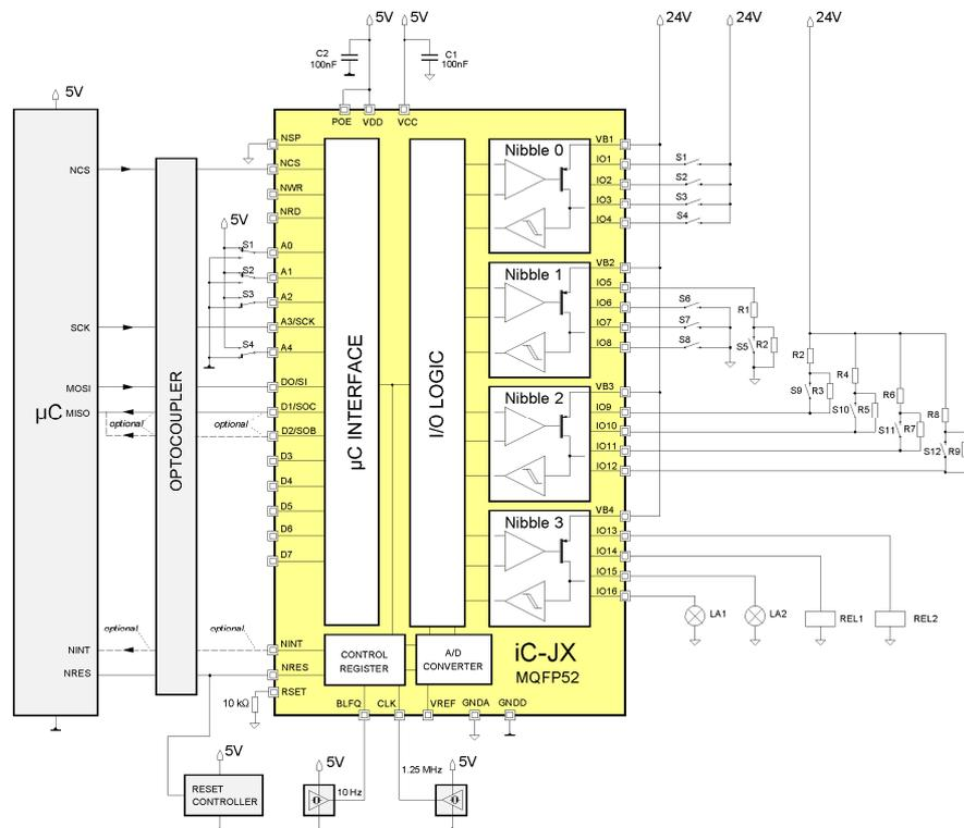
Figure 1: iC-JX in a typical application environment
