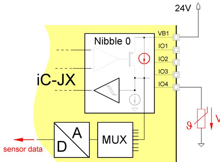
Figure 3: The use of the A/D converter for sensor evaluation
