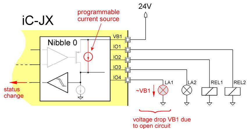
Figure 2: System diagnosis using programmed current sources
