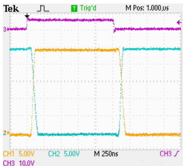
Figure 1: Example of moderate slew rate with un-loaded Ox and NOx outputs ( V_B = 24\text{ V} )
