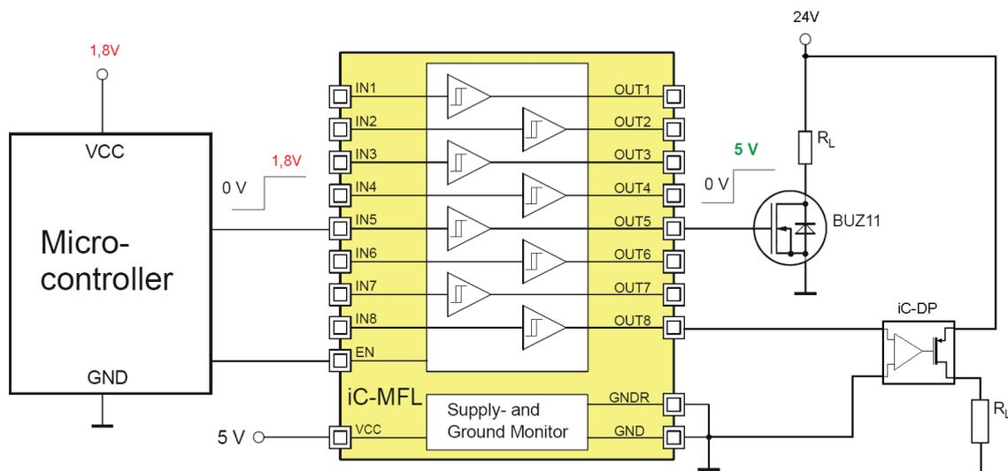
Figure 1: Shifting voltage level and driving power outputs
