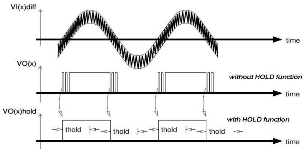
Figure 3: Integrated solution to filter noisy input signals
