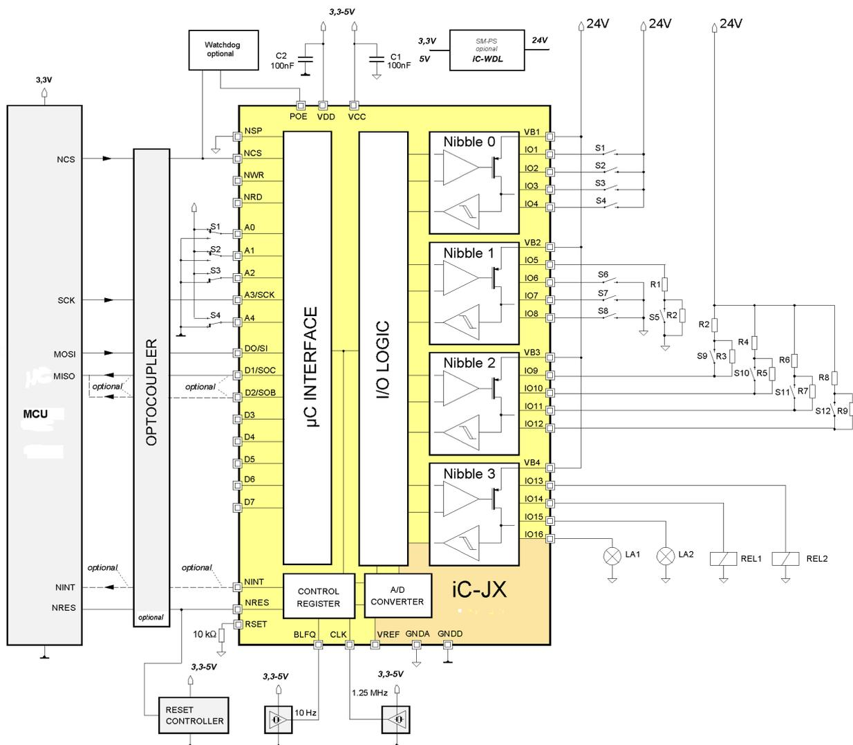
Figure 2: Compact universal I/O with optional isolation
