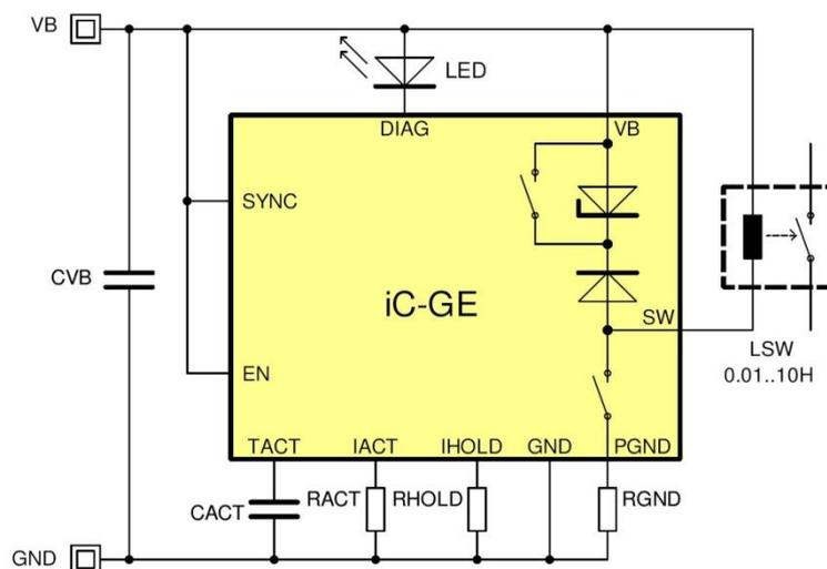
Figure 5: Integrated drive solution to save power consumption in relays or valves
