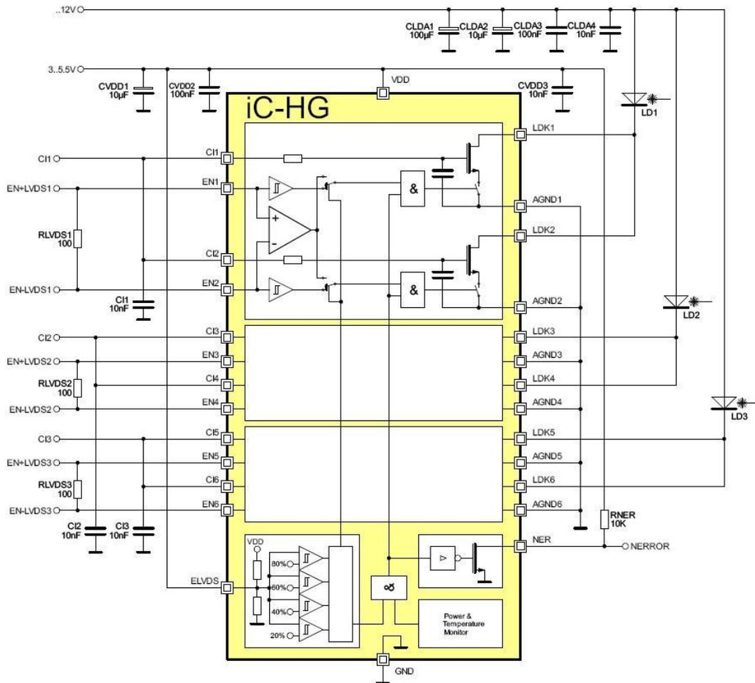
Figure 4: Driving RGB Laser Diodes/LEDs up to 1Amp
