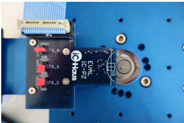
Figure 2: Scanner module (iC-PZ2656 EVAL PZ1M) and code disc PZ03PS in detail
