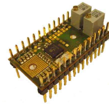
Figure 1: HG2M Package (DIL28)
